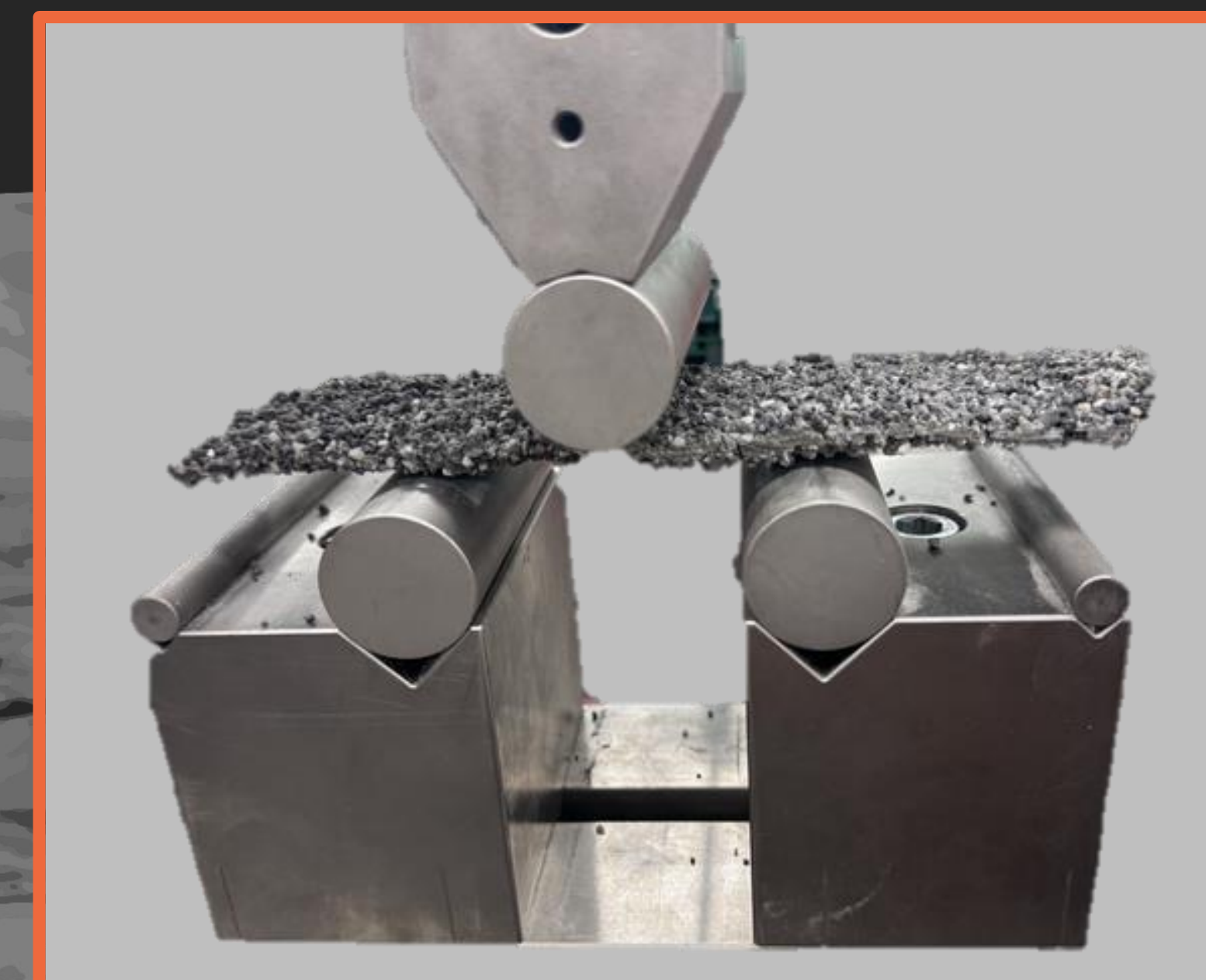
Figure 4: 3-Point Bending Test
